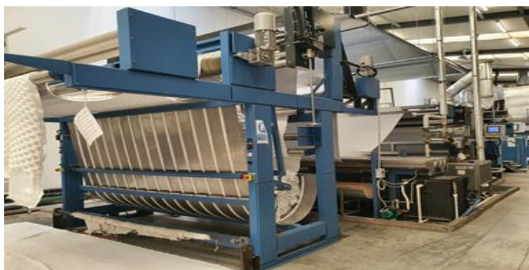
Fig. 1: Equipment for the treatment of textile materials - Squeezing Pader Machine
